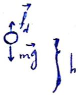
۶  $mg - f_d = ma \Rightarrow a = \frac{mg - f_d}{m} = g - \frac{f_d}{m}$
